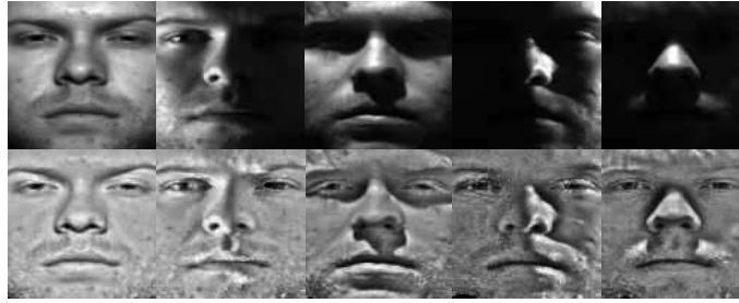
Figure 3.19: Sample images processed with the example code: original images (upper row), LSSF processed images (lower row)
