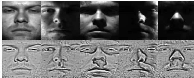
Figure 3.18: Sample images processed with the example code: original images (upper row), MSW processed images (lower row)
