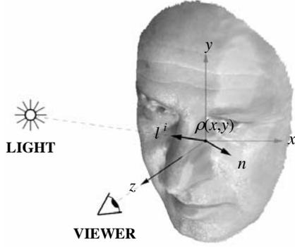
Fig. 1. The photometric stereo acquisition scheme.
